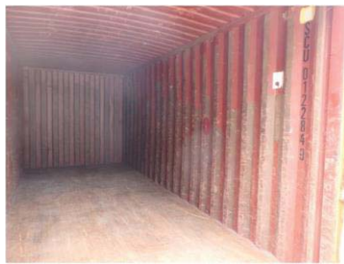
(a) Wall corrugation
