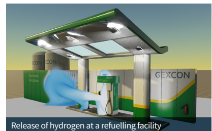
Release of hydrogen at a refuelling facility
