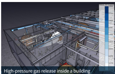
High-pressure gas release inside a building
